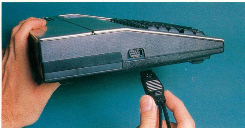
Plug the joystick cable into the Game Controller Port.
